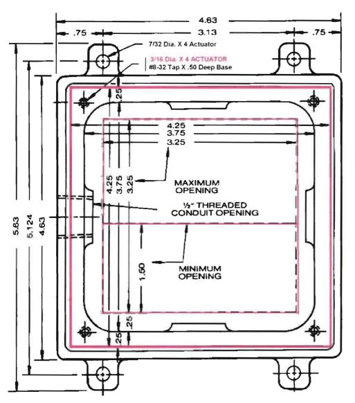
Black Lines Indicate Dimensions for Mounting the M2-BASE.
